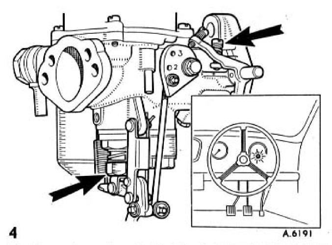
A. Restart the engine and adjust the throttle adjusting screw to give desired idling as indicated by the glow of the ignition warning light.
