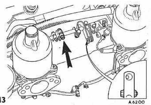
A. Tighten the clamp bolt of the throttle spindle interconnections and set the link pin lever with the pin resting against the edge of the pick-up lever hole (see inset). This provides the correct delay in opening the front carburetter throttle disc.
