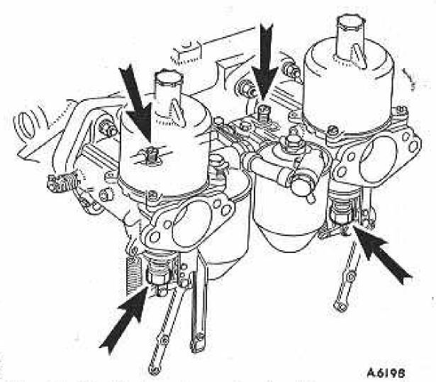
A. Turn the jet adjusting nuts on all carburetters up to weaken or down to richen the same amount until the fastest idling speed consistent with even running is obtained.
