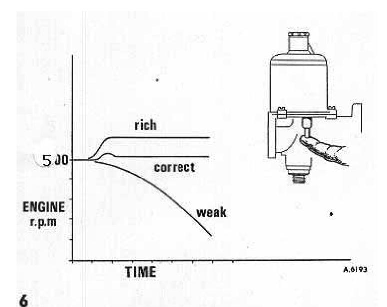
A. Check for correct mixture by gently pushing the lifting pin up about ½ in. (·8 mm.).
